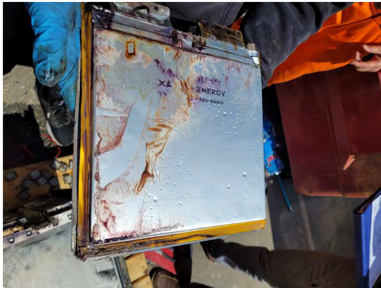
Picture 18 – Unit BBU – Unit After Exposure at 950°C – Back Protection Panel and Insulation Removed – Cell No.24 Back View
