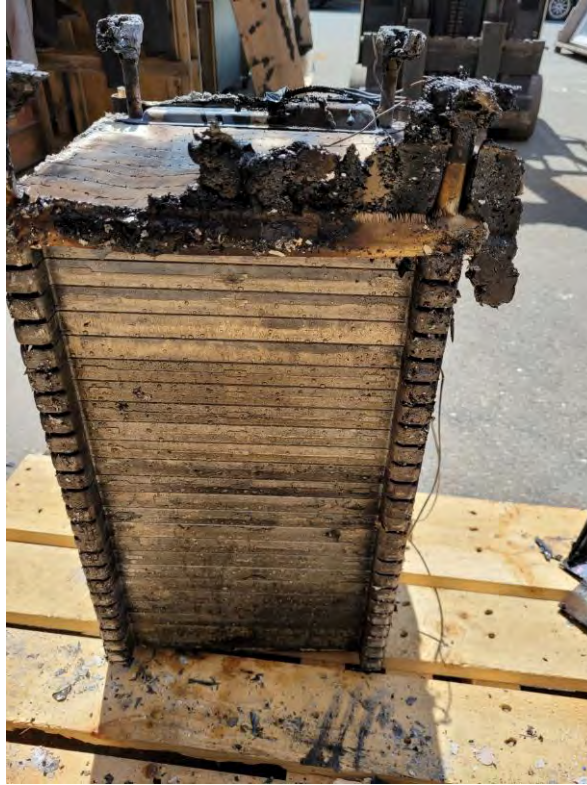
Picture 13 – Unit BBU – Unit After Exposure at 950°C – Battery Only – Bottom View
