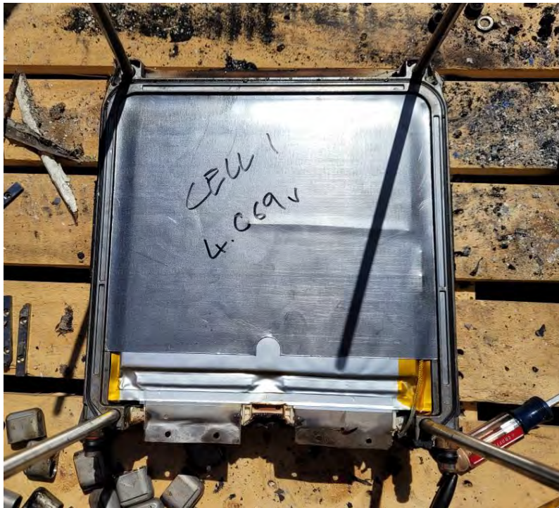
Picture 20 – Unit BBU – Unit After Exposure at 950°C – Cell No.1 View
