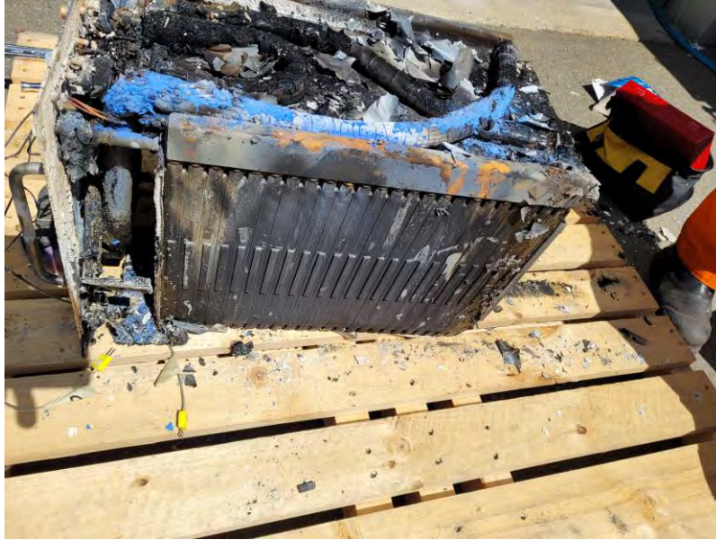
Picture 11 – Unit BBU – Unit After Exposure at 950°C – Battery Only – Side View
