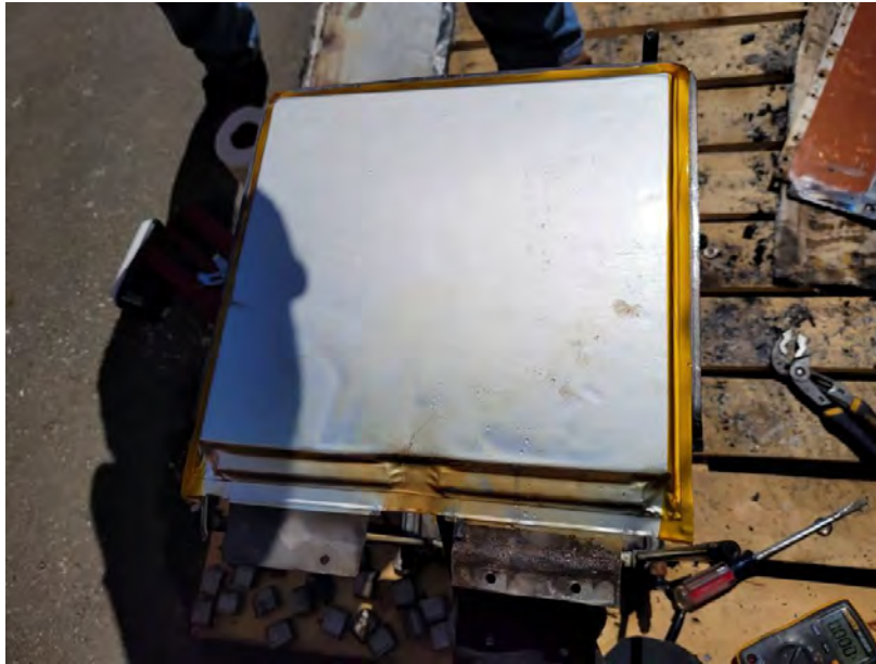
Picture 21 – Unit BBU – Unit After Exposure at 950°C – Cell No.1 Exposed Side View
