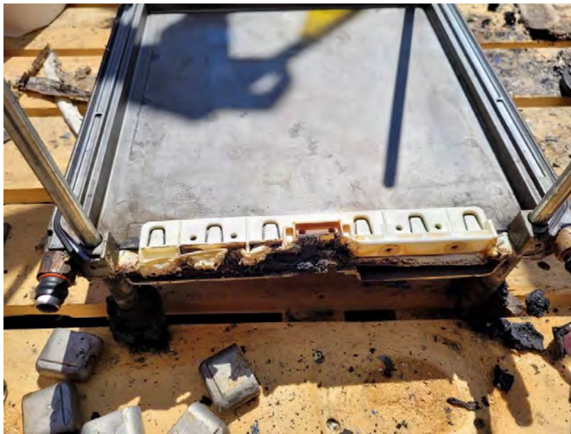
Picture 22 – Unit BBU – Unit After Exposure at 950°C – Front Panel Isolation Block Condition and Close-up of Gas Gasket
