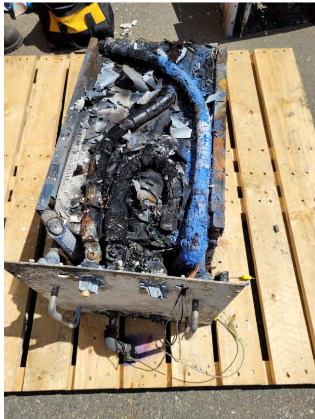
Picture 10 – Unit BBU – Unit After Exposure at 950°C – Battery Only – Top View
