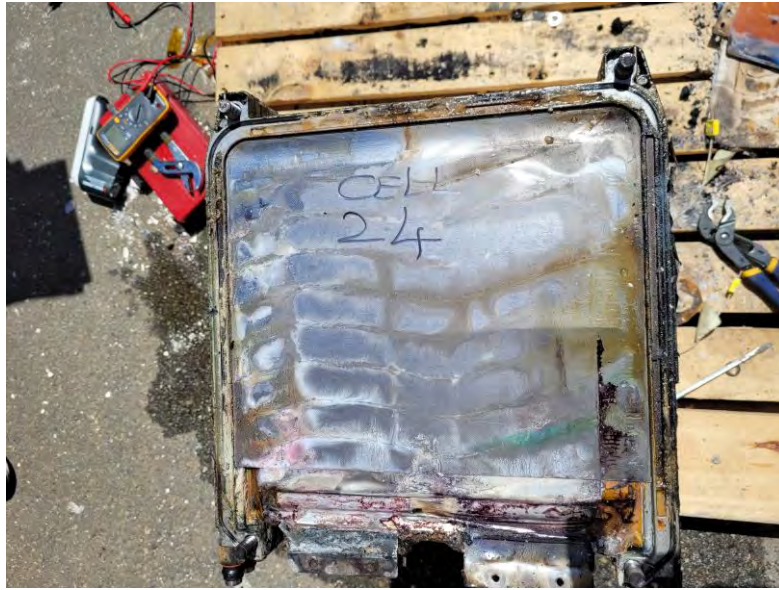
Picture 17 – Unit BBU – Unit After Exposure at 950°C – Back Protection Panel and Insulation Removed – Cell No.24 View
