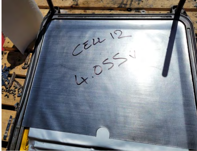
Picture 19 – Unit BBU – Unit After Exposure at 950°C – Cell No.12 View
