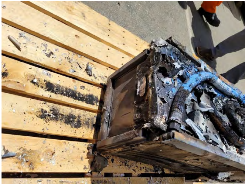
Picture 12 – Unit BBU – Unit After Exposure at 950°C – Battery Only – Back View
